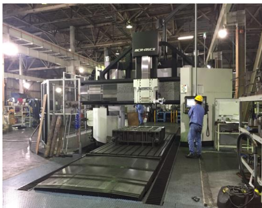
Five-faced processing machine O-KUMA MCR-A5C II 2,500×4,000mm
