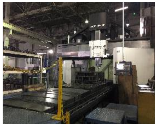
Five-faced processing machine O-KUMA MCR-A5C II 2,000×4,000mm
